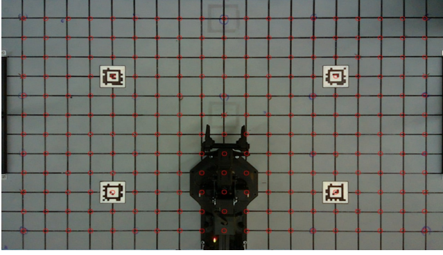
Fig. 7: Grid point projection with homography transform applied
